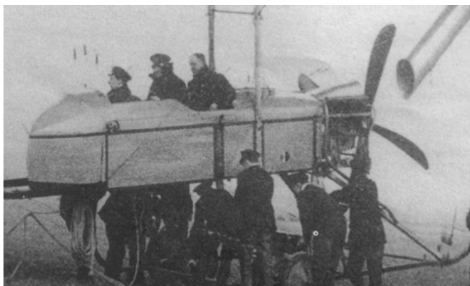
The SS Llangefni Pig were augmented by the SSP with a larger envelope and a more powerful engine. The 'P' stood for pusher. The car used here is a modified Maurice Farman fuselage with the engine in 'pusher' mode. The crew consisted of a pilot, wireless operator/air gunner and an engineer
